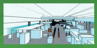
The 3D RF propagation simulations of the 20,000 square metre Smart Factory provided significant advantages when determining the number of base stations required, the preferred locations and the appropriate antenna tilt, with proper attention paid to vital restrictions on where the base stations could be installed.
