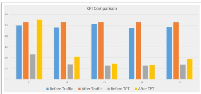
The throughput performance improved by up to 240%, with an average of 50% despite there being higher traffic loading increased pressure on the network. The average user throughput of the overall cluster saw an **improvement of 25%-30%**. This is equivalent to adding 1-2 carriers to the venue which could have cost the Operators millions of dollars to achieve.
